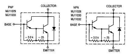
Figure 1. Darlington Circuit Schematic
